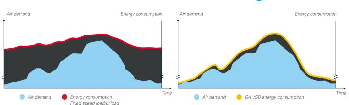
In almost every production environment, air demand fluctuates depending on different factors such as the time of the day, week or even month. Extensive measurements and studies of compressed air demand profiles show that many compressors have substantial variations in air demand. Only 8% of all installations have a more stable air demand.
